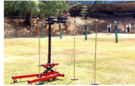
Fig. 8. The configuration of sound intensity measurement in the field
